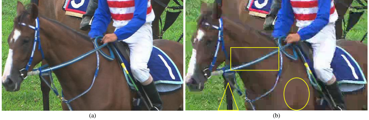
Figure 3. An example of blocking artifacts. (a) Reference frame; (b) Compressed frame with three types of blocking artifacts: mosaic effect (elliptical region); staircase effect (rectangular region); false edge (triangular region).
