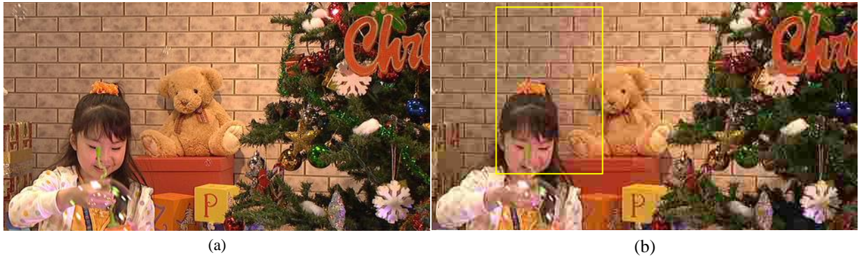
Figure 6. An example of color bleeding artifact. (a) Reference frame; (b) Compressed frame with color bleeding.
