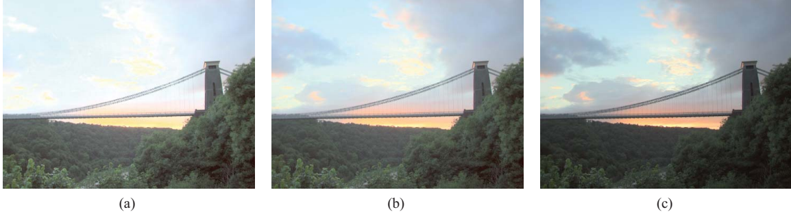
Fig. 7. LDR images generated with different parameter b in (17). (a) b = 0.1 , S = 0.5214 , N = 0.0249 , and Q = 0.7535 . (b) b = 0.7 , S = 0.8137 , N = 0.1136 , and Q = 0.7690 . (c) b = 1.0 , S = 0.8856 , N = 0.2923 , and Q = 0.7967 .
