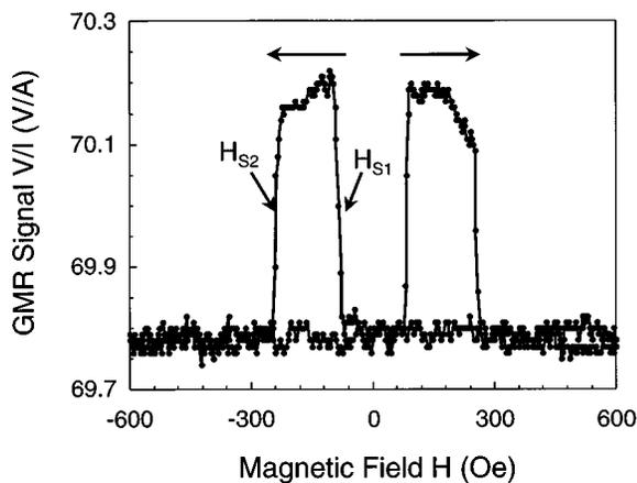
FIG. 3. GMR curve of patterned spin-valve bar of  $300\text{ nm} \times 3\text{ }\mu\text{m}$ , where  $H_{s1} = 85\text{ Oe}$  and  $H_{s2} = 240\text{ Oe}$ . The pattern was fabricated by ion milling.
