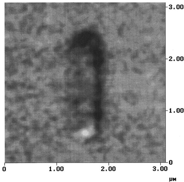
FIG. 5. MFM image of patterned spin-valve bar of  $150\text{ nm} \times 2\text{ }\mu\text{m}$  without leads by ion milling. Two opposite magnetic poles at bar ends indicate the formation of single domain.
