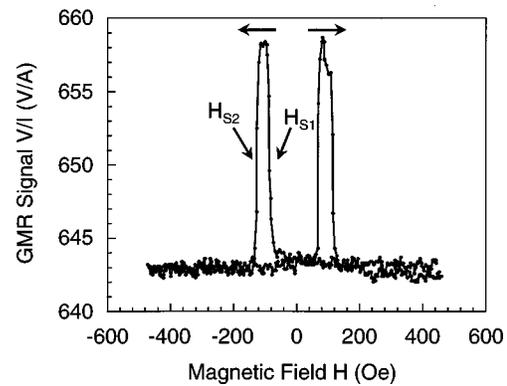
FIG. 7. GMR curve of spin-valve bar patterned by lift-off process. The bar size is  $100\text{ nm} \times 3\text{ }\mu\text{m}$ . In the figure,  $H_{s1} = 85\text{ Oe}$  and  $H_{s2} = 125\text{ Oe}$ .
