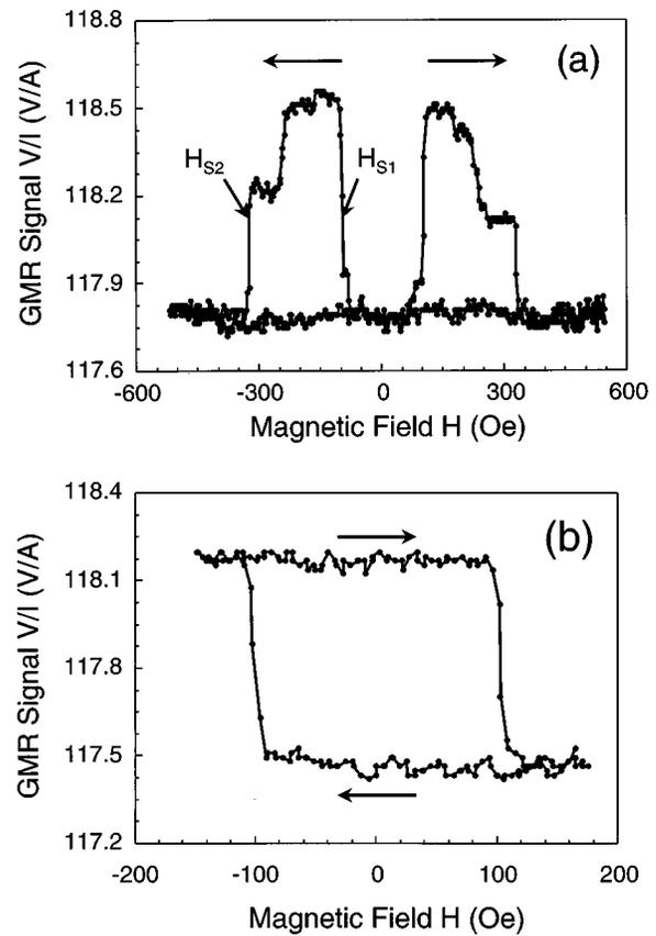
FIG. 4. (a) GMR curve and (b) minor loop of patterned spin-valve bar of  $200\text{ nm} \times 3\text{ }\mu\text{m}$  by ion milling. In Fig. (a),  $H_{s1} = 100\text{ Oe}$  and  $H_{s2} = 325\text{ Oe}$ .
