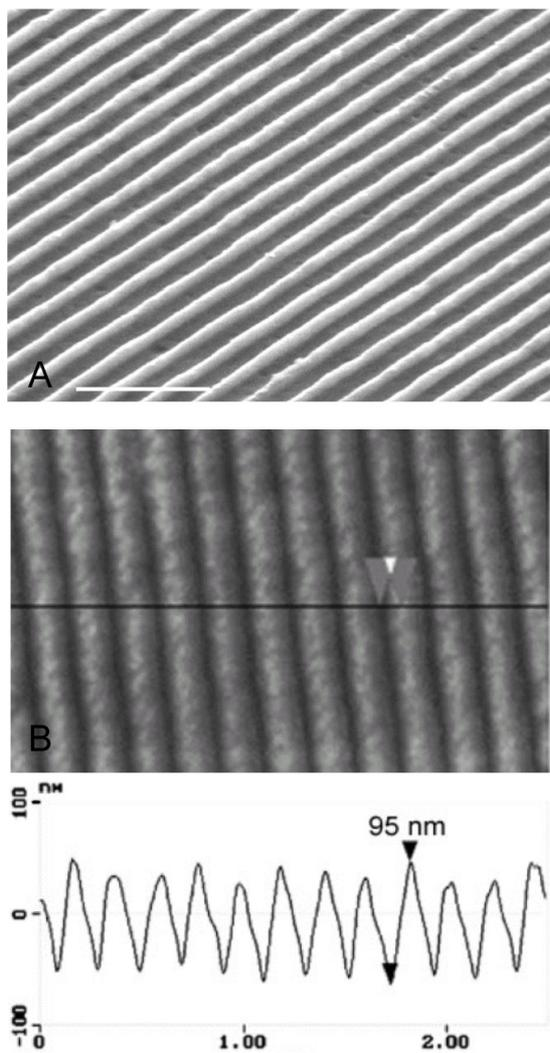
**Figure 2.** A 200 nm period Ni grating patterned by LADI with laser irradiation from the substrate at laser fluence of  $0.60 \text{ J cm}^{-2}$ . (A) SEM image; (B) AFM (atomic force microscope) image showing an average trench depth of 90 nm with about 10 nm fluctuation, close to the trench depth on the mold (100 nm). Scale bar is  $1 \mu\text{m}$ .
