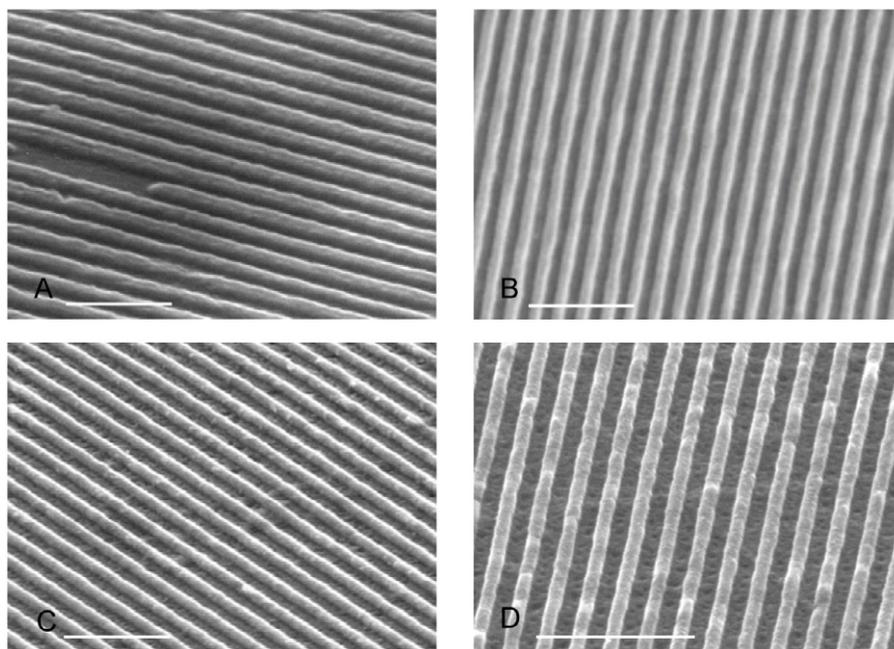
**Figure 1.** SEM images of 200 nm period metal gratings patterned by LADI. (A) Al, laser fluence  $0.22 \text{ J cm}^{-2}$ ; (B) Au,  $0.53 \text{ J cm}^{-2}$ ; (C) Cu,  $0.24 \text{ J cm}^{-2}$ ; (D) Ni,  $0.41 \text{ J cm}^{-2}$ . Scale bar is  $1 \mu\text{m}$ .
