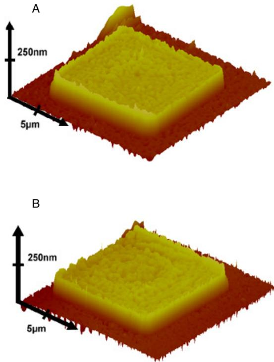
**Figure 4.** AFM image of isolated mesas patterned by LADI. The mesas have a length on each side of  $17 \mu\text{m}$ , and a height of  $100 \text{ nm}$ . (A) Au, laser fluence  $0.45 \text{ J cm}^{-2}$ ; (B) Cu,  $0.45 \text{ J cm}^{-2}$ . (This figure is in colour only in the electronic version)
