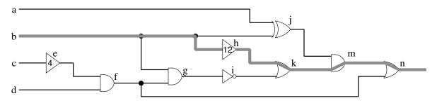
1. Prelude: check longest path (not needed in real solution, because we are told that this is a false path.)
