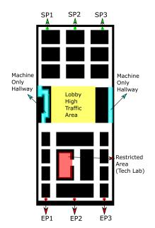
Fig. 1: Map of the target environment. Empty space is in white and occupied space is in black. The green dots represent the 3 possible starting locations while the red dots represent the 3 possible end locations. The central empty area is the "Lobby" of the warehouse, while the two hallways to the left and right of the "Lobby" are machine only areas.
