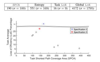
Fig. 5: Average LOE versus SPCA. In this figure, the average LOE was calculated over the 9 pair of start and end points that specified the robot task.
