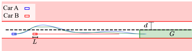
Fig. 7: This figure shows the trajectories generated in robust mode with N = 10 waypoints, comparing the baseline (green) and proposed (blue) trajectories. Here, the robustness achieved for both the trajectories is the same. An animation viewed here: To view an animation, visit here: https://youtu.be/1953Gh-BBSI
