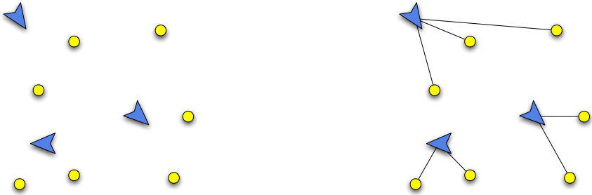
Figure 1.1: An illustration of task allocation. Vehicles are denoted by chevrons, and task locations by disks. The left-figure shows a group of vehicles and a set of tasks and the right-figure shows an allocation of tasks to vehicles.
