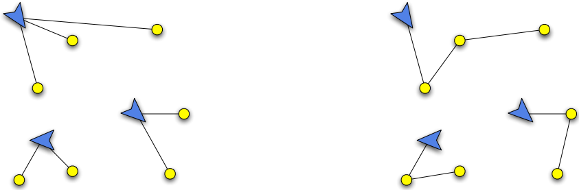
Figure 1.2: An illustration of vehicle routing. Vehicles are denoted by chevrons, and task locations by disks. The left-figure shows a task allocation and the right-figure shows a set of routes for completing the tasks.
