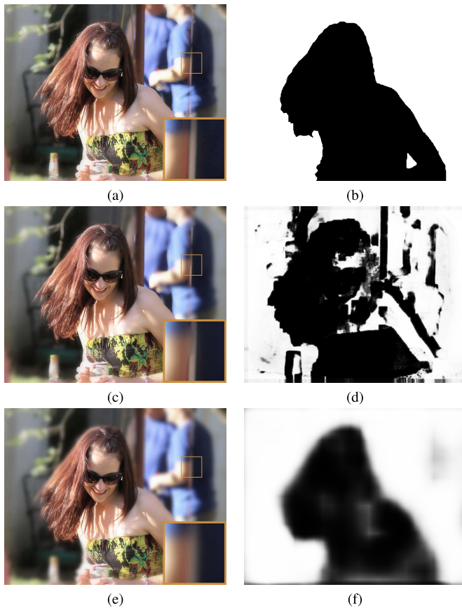
Fig. 12. The blur magnification results. (a) Test image from the blur detection benchmark [11]. (b) Ground truth blur map. (c) Magnification by Shi14 [11]. (d) Blur map by Shi14 [11]. (e) Magnification by DBM. (f) Blur map by DBM.
