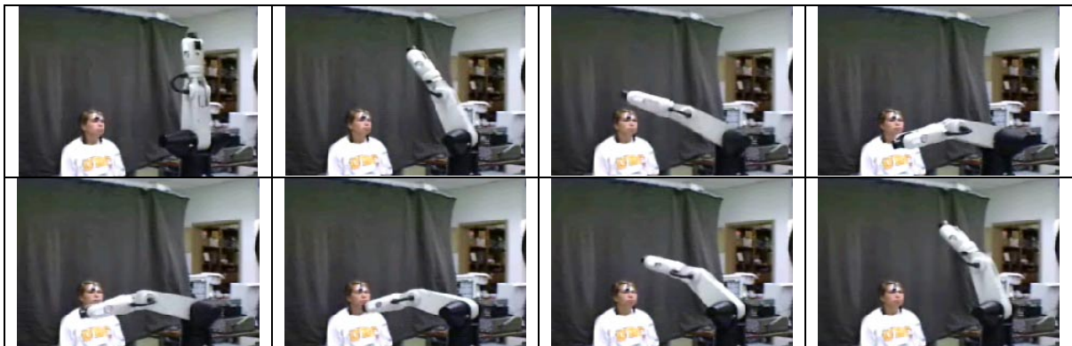
Figure 6.5. Path PP-PF (pick and place task planned with the potential field planner).
