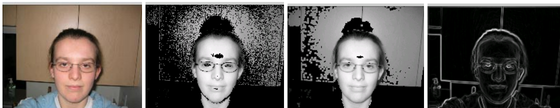
Figure 6.17. Face detection with skin coloured background.
