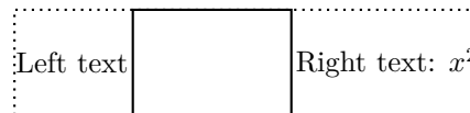
Figure 61: The macro s_box sets string dimensions automatically when processed twice. If two or more arguments are given to s_box , they are passed through sprintf . The dots show the figure bounding box.
