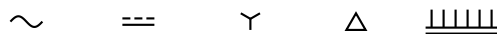
Figure 46: The elements ACsymbol , DCsymbol , Ysymbol , Deltasymbol , and heatsink(at position, keys, U|D|L|R|degrees) have similar argument sequences.
