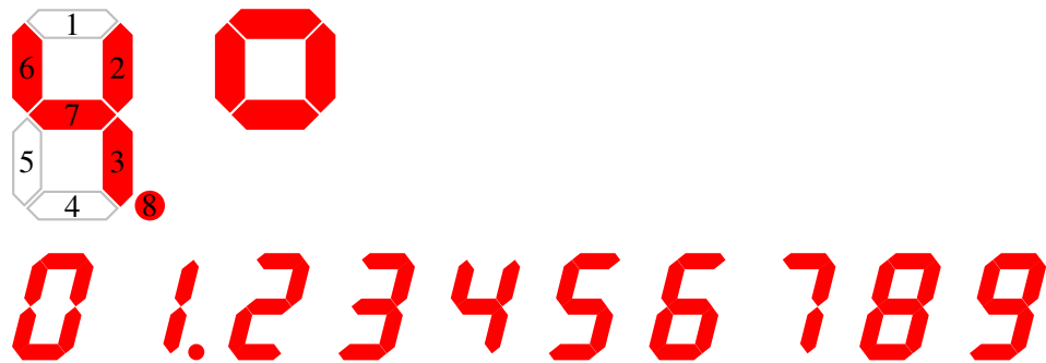
Figure 97: A customizable seven-segment display showing the numbered segments, a custom shape, and the numerals from 0 to 9 [Sevensegment.m4].
