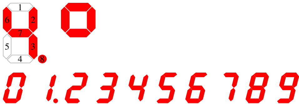
Figure 88: A customizable seven-segment display showing the numbered segments, a custom shape, and the numerals from 0 to 9 [Sevenssegment.m4].
