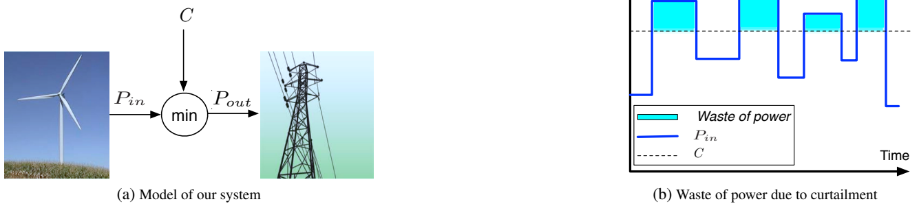
Figure 2: A simple model for curtailment: when a renewable energy source produces more power than can be carried on a transmission line of capacity C , the excess is wasted.
