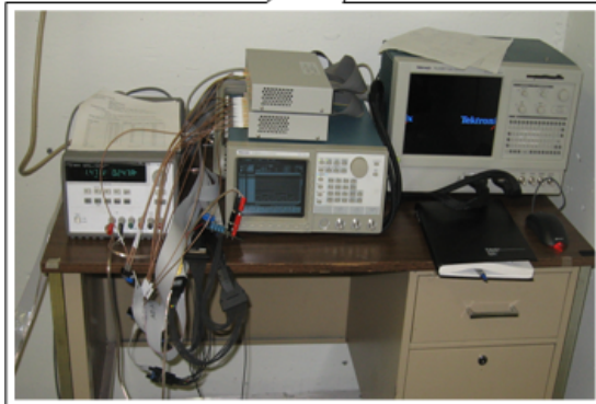
Test equipment monitoring the SRAM SER
