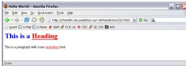
Figure 12. An additional style colouring all underlined text red.
