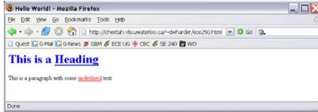
Figure 13. Only underlined text within paragraphs is coloured red.
