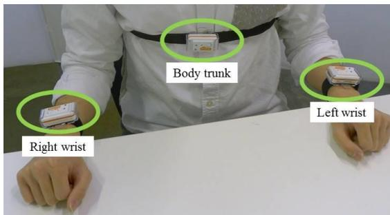
Figure 1. Attached position of 3 IMU sensors.
