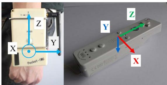
Fig. 2. IMU and Wii Remote axial directions.
