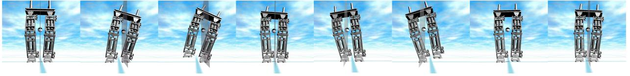
Fig. 6. Frames from the sequence of motions while side stepping. The gray plane in the frame captures above represents the 2D FPE plane which moves along the Y-direction (biped’s frontal plane). The intersection of the gray 2D FPE plane and the ground plane indicate the FPE point tracked during **DROP**.
