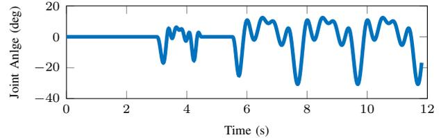
Fig. 5. Simulation of complex human motion. First, three seconds are used as the static interval. Next, a single motion repetition is generated as a sum of five sinusoids with random coefficients. The movement is paused from 4.5 to 5.5 seconds. Finally, three more movement repetitions are completed at double magnitude and half the frequency of the first.
