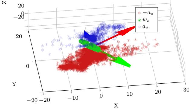
Fig. 10. 3D scatter plot of the accelerometer (blue), its rotated set symmetric about origin (red) and gyroscope (green) data during gait. Note only every fifth  $a_{imu}$  point is plotted to better see the gyroscope signal. The red and green arrowheads show the actual components of the rotation matrix. It is clear that the gyroscope principal direction is well aligned with  $s_{x_0}$ .
