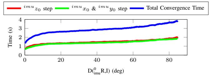
Fig. 4. Convergence times of the  ${}^s z_0$  estimation (red),  ${}^s x_0$  and  ${}^s y_0$  (green) steps and total time (blue) at different sensor orientations. After a rotation offset of larger than 10 deg a linear increase in convergence time is observed.
