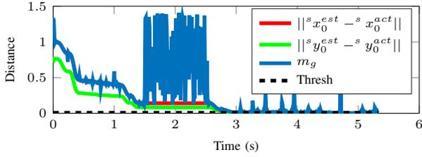
Fig. 6. Convergence of the  ${}^s x_0$  and  ${}^s y_0$  components during complex motion. The algorithm successfully converges on an accurate estimate of the components and does not update them during a pause in the movement, when gyroscope noise dominates the signal. After 6.5 seconds the  ${}^s x_0$  and  ${}^s y_0$  components are estimated with  $2.1 \times 10^{-3}$  and  $8.2 \times 10^{-4}$  error norms respectively.
