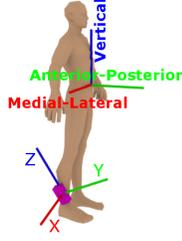
Fig. 1. The human body and IMU frames for a shank worn IMU.
