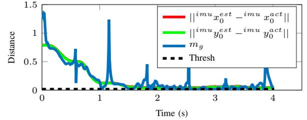
Fig. 8. Estimation of the  ${}^s x_0$  and  ${}^s y_0$  components during knee flexion-extension. Unlike the accelerometer, the gyroscope has significantly better alignment to the axes defined by the markers placed on the IMU and the  ${}^s x_0$  and  ${}^s y_0$  are accurately estimated with 0.048 and 0.041 error norms respectively.
