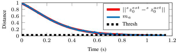
Fig. 2. Convergence of the  ${}^s z_0$  component when the sensor is rotated 45 deg in roll, pitch, and yaw with respect to the link frame. Note that while the convergence metric  $m_a$  (blue) is susceptible to sensor noise the distance between actual and estimated  ${}^s z_0$  components converges smoothly to zero. After only 1.2 seconds 20 samples fall below the convergence metric standard deviation threshold (black), the algorithm terminates with a final error of  $2.5 \times 10^{-3}$ .
