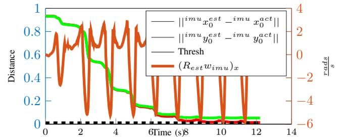
Fig. 9. Convergence of the  ${}^s x_0$  and  ${}^s y_0$  components during natural gait. After applying the estimated rotation to the gyroscope measurement we plot the angular velocity of the medial-lateral axis, the components converge in only 9 gait cycles.
