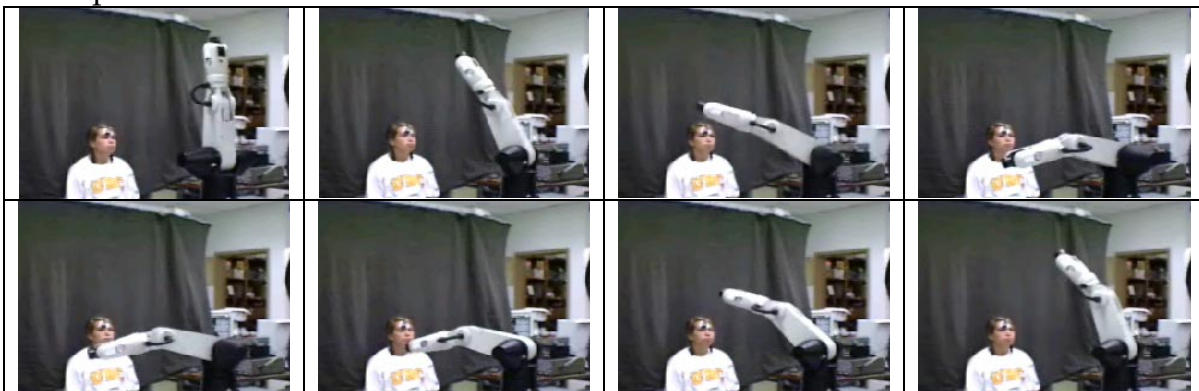
Figure 11 - Path PP-PF (Pick and Place Task Planned with the Potential Field Planner)
