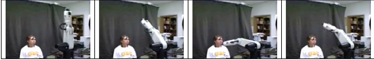
Figure 13 - Path RR-PF (Reach and Retract Task Planned with the Potential Field Planner)
