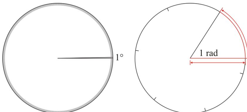
Figure 6. Definitions of the degree and the radian.
