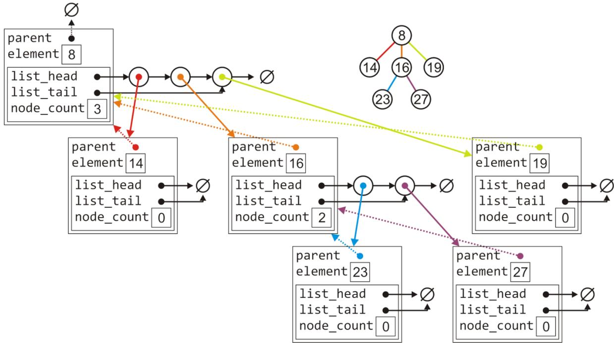
Figure 1. A tree of six nodes stored in the `Simple_tree` data structure.
