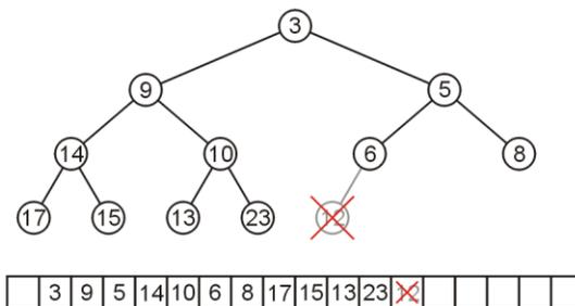
Figure 5. Removing a node from a complete tree.
