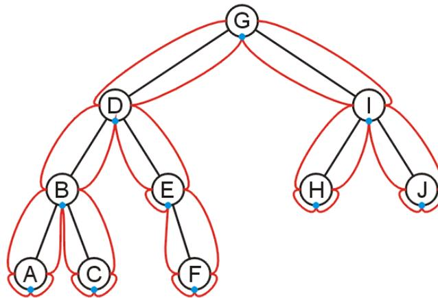
Figure 1. An in-order traversal of a binary tree.
