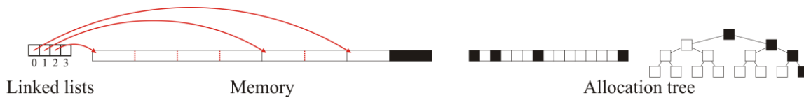
Figure 5-9. The state of our memory allocation scheme after one block of size K was allocated.
