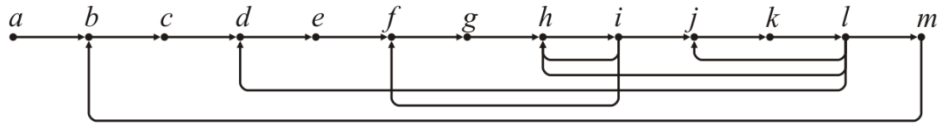
Figure 11-8. The directed graph of a block diagram of a position servo with multi-loop feedback.
