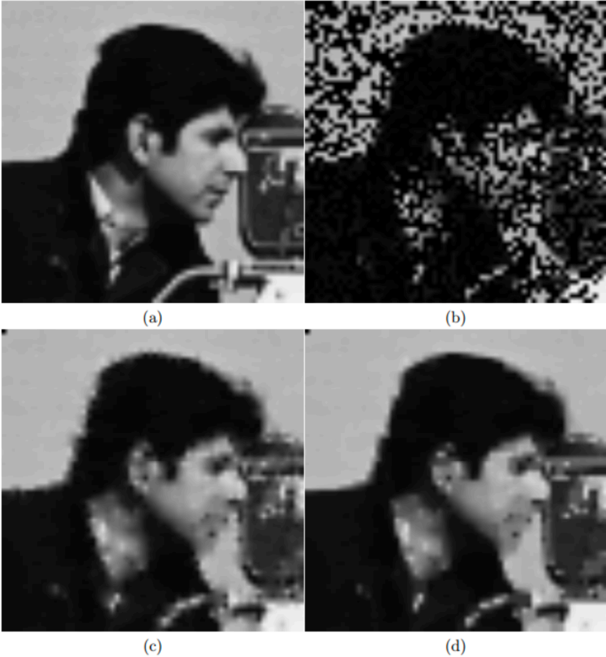
Figure 1: Image Interpolation. (a) Original image. (b) Obscured image. (c) \ell_2 reconstructed image. (d) TV reconstructed image.
