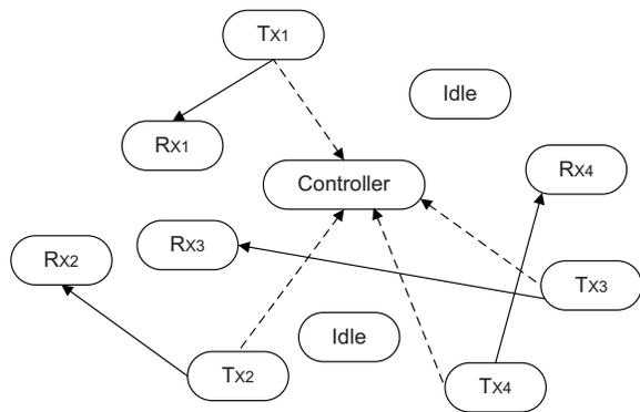
Fig. 1. Indoor mmWave Network Architecture
