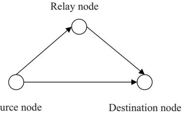
Fig. 3. Three-Node Model for Cooperative Communication
