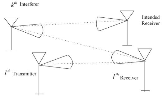
Fig. 9. Geometry of directional interference.
