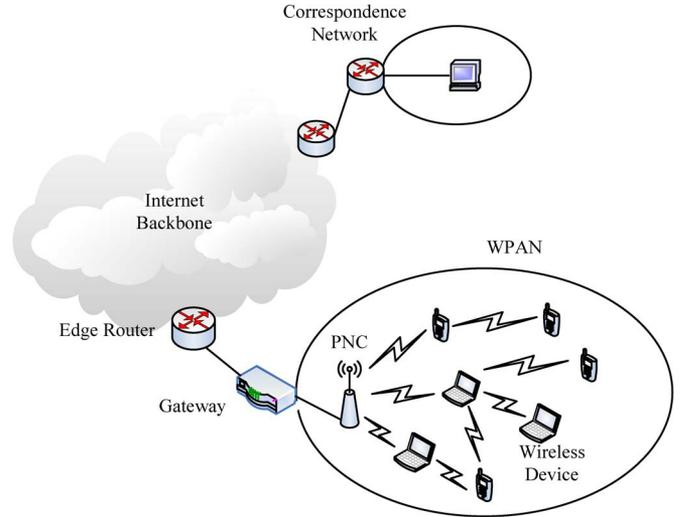
Fig. 1. Indoor mmWave network architecture.
