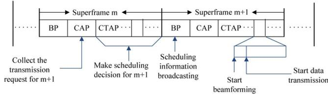
Fig. 4. Procedure for scheduling and beamforming.
