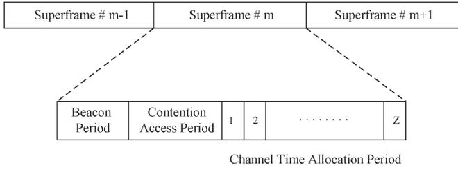
Fig. 2. Superframe-based timing structure.
