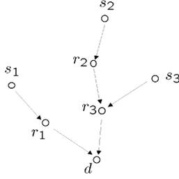
Fig. 6. A multisource single-sink sensor network.
