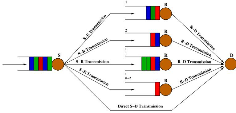
Figure 4: Network model for a particular S-D pair. The source queue is a simple Bernoulli( $\lambda$ )/Bernoulli( $\frac{\phi}{2}$ ). Each packet either goes directly to the destination or through one of the  $n - 2$  relay nodes. The relay queues are GI/GI/1-FCFS.
