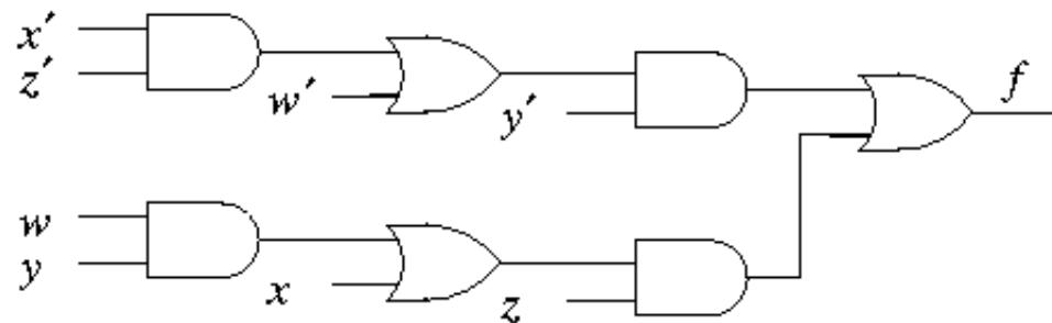
insert inverter bubbles and replace with NANDs
