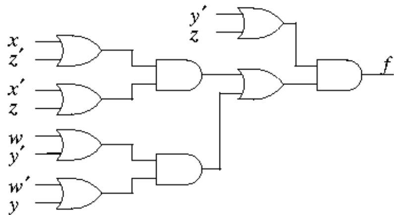
Insert inverter bubbles and convert to NOR gates:
