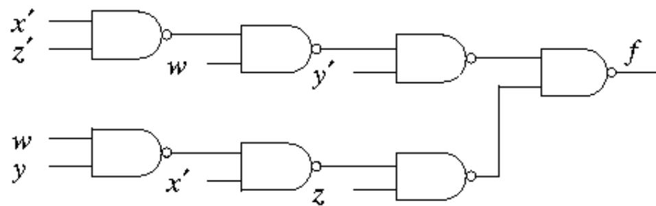
NB: Note inputs to third level have been complemented compared to AND-OR-AND-OR circuit.
