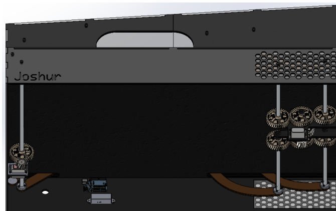
Figure 7: Underside of VTOL dock, with the two gear trains visible on either side, and Arduino in bottom middle.
