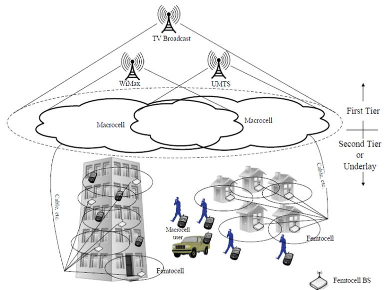
Fig. 1: Femtocell underlay in the two-tier architecture.
