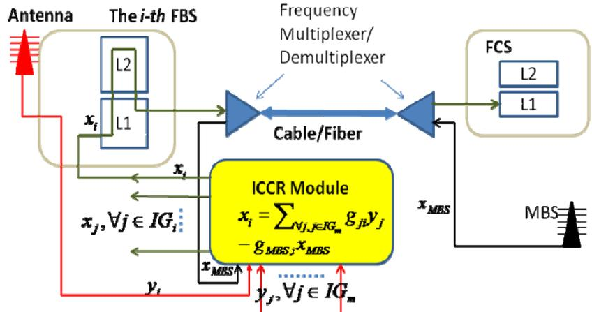
Fig. 5. Diagram for the proposed distributed WOC architecture.
