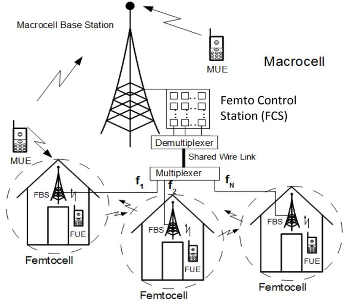
Fig. 2. An illustration of femtocell network architecture.
