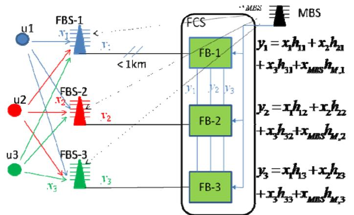
Fig. 3. A diagram of the WOC architecture. The signals ( $y_i$ ) along the cables/fibers are due to the interferences from adjacent FBSs and the MBS.
