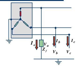
The terminal unbalance currents at the fault point can be transferred into their sequence components as follows:
