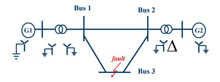
For the generators assume  $Z^+ = Z^- = j0.2$ ;  $Z^0 = j0.05$ For the transformers assume  $Z^+ = Z^- = Z^0 = j0.05$ For the lines assume  $Z^+ = Z^- = j0.1$ ;  $Z^0 = j0.3$ Assume unloaded pre-fault, with voltages =1.0 p.u.
