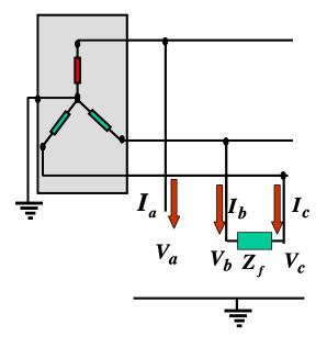
Current relationships:  $I_a = 0$  &  $I_b = -I_c$ Voltage relationships:  $V_b = V_c + I_b Z_f$
