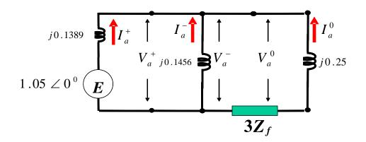
$$V_{a}^{+} = 1.05 - 4.547 \angle -90^{\circ} \times j0.1389 = 0.4184$$
