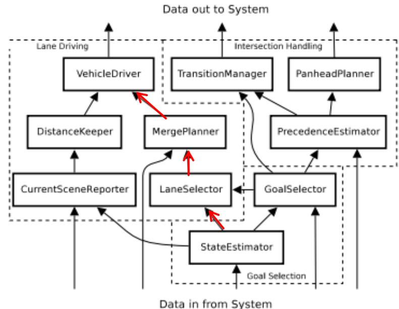
Figure 14. High-level behaviors architecture.
