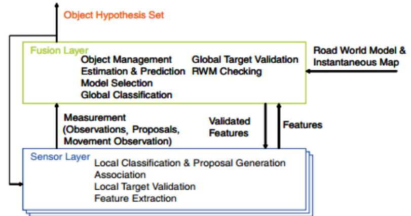
Figure 8. The moving obstacle detection and tracking system architecture.
