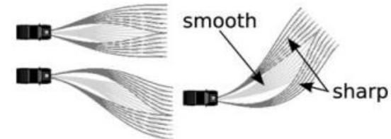
Figure 4. Smooth and sharp trajectories. The trajectory sets are generated to the same endpoints but differ in their initial commanded curvature.
