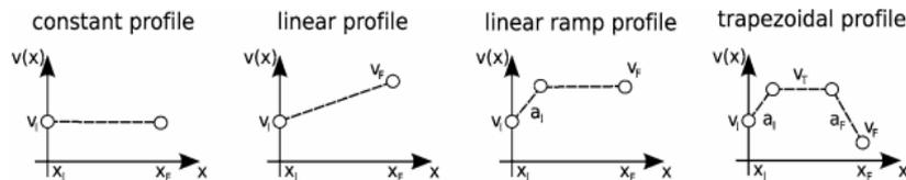
Figure 3. Velocity profiles used by the trajectory generator.
