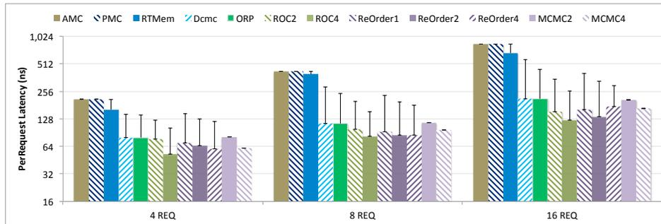
Fig. 5: WC Latency per Close Request of REQ0 with 64Bit Data Bus.
