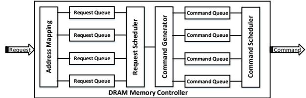
Fig. 1. Generalized Real-Time Memory Controller Architecture.
