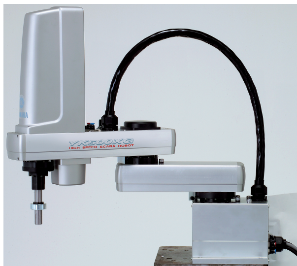
Figure 3.14: The Yamaha© YK500XG is a high-speed SCARA robot with two revolute joints and a vertical prismatic joint. Image courtesy of Yamaha Motor Co., Ltd, http://global.yamaha-motor.com/business/robot .
