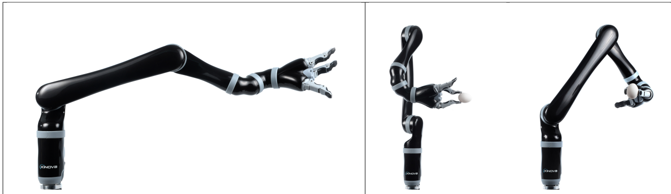
Figure 8.4: The Jaco 2 by Kinova Robotics is a light-weight robot arm with six degrees of freedom. Images courtesy of Kinova Robotics, http://kinovarobotics.com/ .
