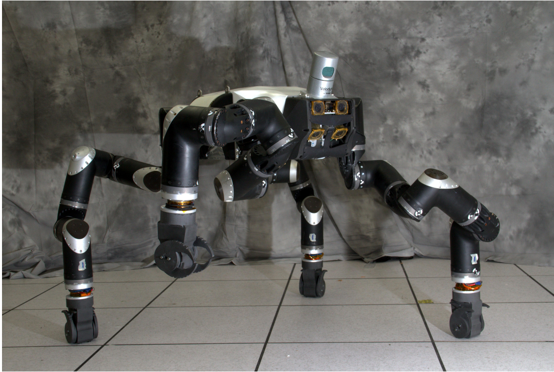
Figure 3.3: RoboSimian is an ape-like robot that moves around on four limbs. It was designed and built at NASA's Jet Propulsion Laboratory in Pasadena, California. It will compete in the 2015 DARPA Robotics Challenge Finals. Image courtesy of NASA/JPL-Caltech.
