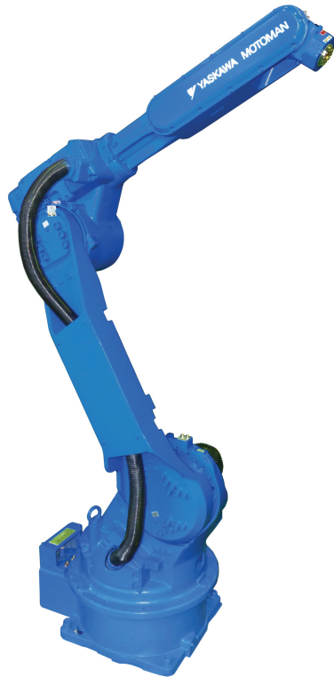
Figure 3.2: The Motoman® HP20 manipulator is a multi-body robot versatile high-speed industrial robot with a slim base, waist, and arm. Image courtesy of Yaskawa Motoman, http://www.motoman.com .
