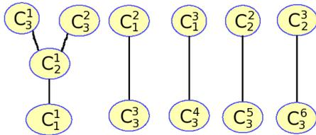
Fig. 4: Example of a collision graph used to construct the collision zones  $CZ^m$ . In this graph, there are 12 nodes corresponding to the disjoint connected sets in  $P_1, P_2, P_3$ , for robots 1, 2 and 3, respectively. The result from this graph is that there are five disjoint collision zones, i.e.  $CZ^m, m \in \{1, 2, 3, 4, 5\}$ . These five collision zones are mapped to their respective paths in Figure 3.
