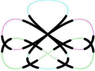
Fig. 3: Plot of paths for the three robots, whose collision zones were obtained in Figure 4. The final five collision zones  $CZ^m$  are plotted in segments of black, while the rest of the trajectories are plotted in different light colors.
