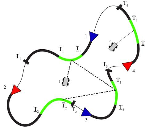
Fig. 2. Four working robots (blue and red triangles) traveling along one path. For each working robot  $r$ ,  $[0, T_r]$  is denoted by a bold black line and  $[\underline{T}_r, \bar{T}_r]$ , by a bold green line. The two grey charging robots must meet all working robots on their paths within their charging windows to guarantee persistent operation.
