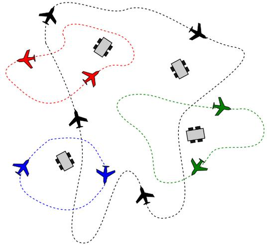
Fig. 1. A persistent monitoring scenario with multiple coordinated UAVs and charging robots. Assuming planar UAV paths, we consider a 2D projection of the environment at ground level.
