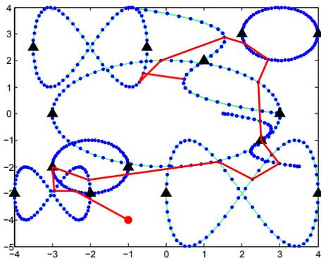
Fig. 7. The heuristic solution (computed using LKH) to the single charging robot problem with sixteen working robots distributed among eight paths.
