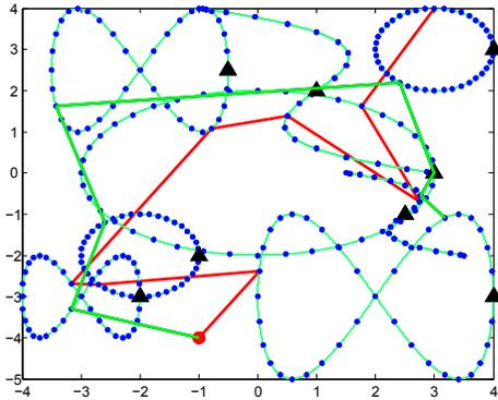
Fig. 6. Comparison of the optimal CPLEX solution (green path) against the heuristic LKH solution (red path). The problem consists of 8 working robots (triangles) on 8 paths.
