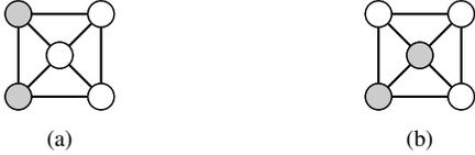
Fig. 2: Example of different solutions of single-stage optimal and infinite horizon optimal solutions. The dark vertices are occupied with the robots. (a) shows the initial configuration and the optimal solution of single-stage. (b) shows the optimal policy for the given initial configuration in infinite horizon.
