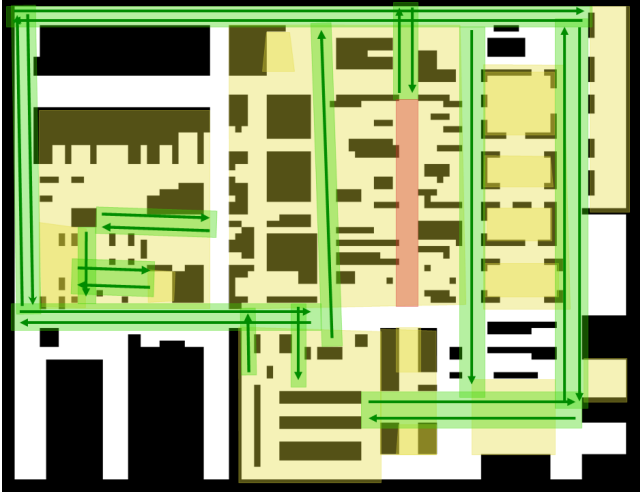
Figure 6. Example specification from participant 5. Reduced speed rules are marked in yellow, road rules in green, and avoidance rules in red.
