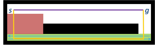
Figure 2. Example for increase in task completion time. The initial specification results in path P^{\text{init}} , shown in purple. An alternative solution (yellow) might have a longer traversal time, but correspond better to the user preferences if they value the avoid zone as less important and prefer the use of the road.
