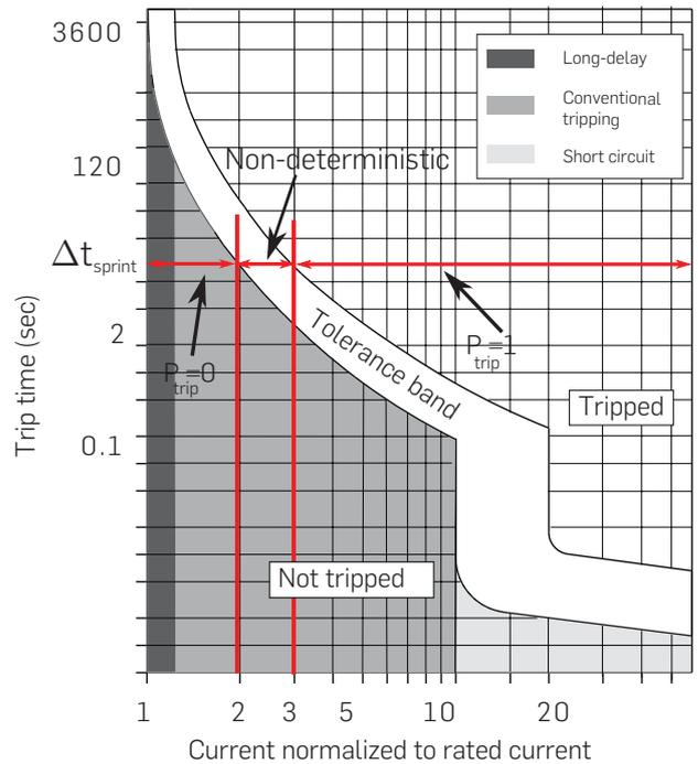
to the number of simultaneous sprints as each sprinter contributes to the load above rated current. Higher currents increase the probability of tripping the breaker.
