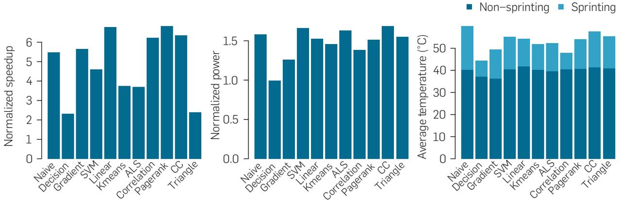
and heat sink must absorb surplus heat during a sprint.<sup>14, 15</sup> Second, the datacenter rack must employ batteries to guard against power emergencies caused by a surplus of sprinters on a shared power supply. Third, the system must implement management policies that determine which chips sprint.
