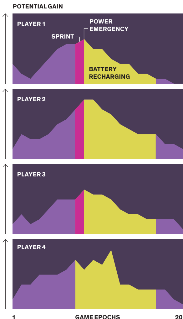
If too many players choose to sprint at once, the increase in current can cause a power emergency. No one, not even player 4, who did not sprint, is allowed to sprint again until the computer cluster’s uninterruptible power supply battery has recharged.
