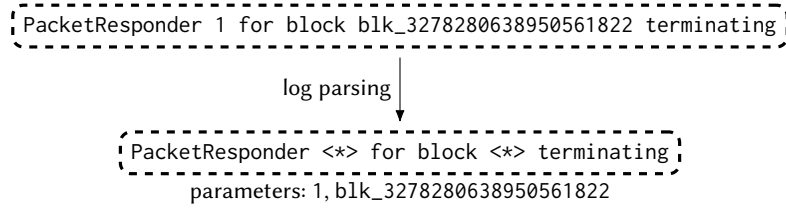
Fig. 1. An example of a log parsing process. The log on the top is parsed into the log template of the bottom.
