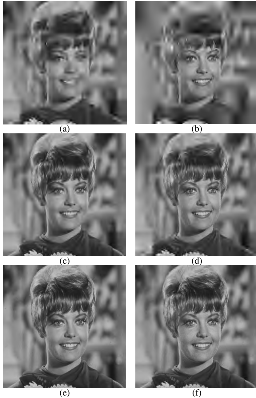
Figure 1.14: “Zelda” image compressed with SPIHT and EFIC algorithms. (a) SPIHT compressed image, compression ratio (CR) = 512:1; (b) EFIC compressed image, CR = 512:1; (c) SPIHT compressed image, CR = 128:1; (d) EFIC compressed image, CR = 128:1; (e) SPIHT compressed image, CR = 32:1; (f) EFIC compressed image, CR = 32:1. (Adapted from [31])
