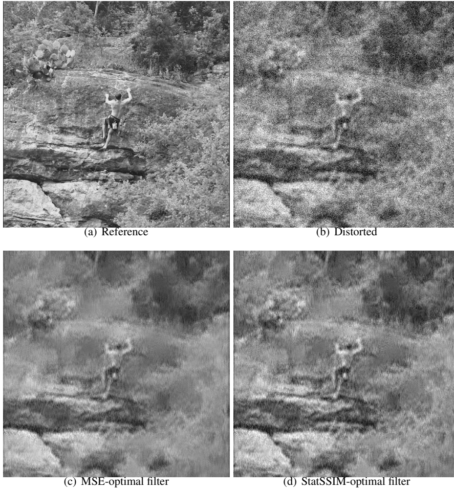
Fig. 6 Restoration example 1: Image Img0073.bmp of the ‘City of Austin’ database. 6(a) Original image. 6(b) Distorted image with \sigma_{blur} = 15 , \sigma_{noise} = 40 , MSE = 2264.4425 , SSIM\ index = 0.3250 . 6(c) Image restored with a 11-tap MSE-optimal filter, MSE = 955.6455 , SSIM\ index = 0.3728 . 6(d) Image restored with a 11-tap SSIM-optimal filter, MSE = 1035.0551 , SSIM\ index = 0.4215 .
