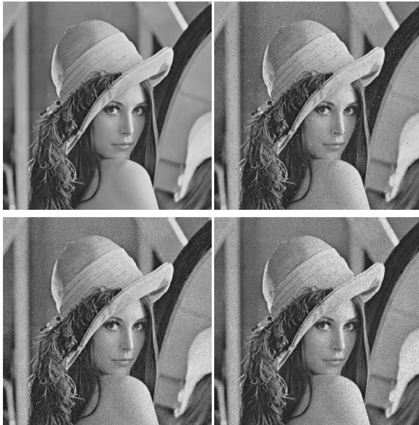
Figure 41.8 Evaluation of “Lena” images with different types of noise. Top-left: Original “Lena” image, 512×512, 8bits/pixel; Top-right: Impulsive salt-pepper noise contaminated image, MSE=225, Q=0.6494 ; Bottom-left: Additive Gaussian noise contaminated image, MSE=225, Q=0.3891 ; Bottom-right: Multiplicative speckle noise contaminated image, MSE=225, Q=0.4408 .
